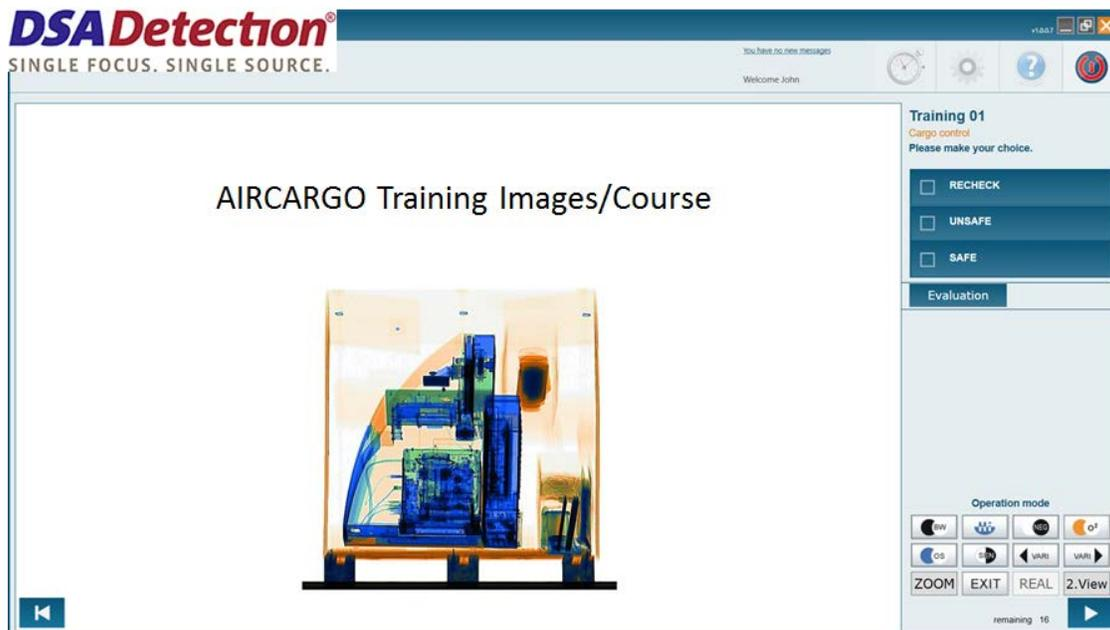
*Figure 8: Air Cargo-based CBT depicting X-ray image of shipping box on pallet*
